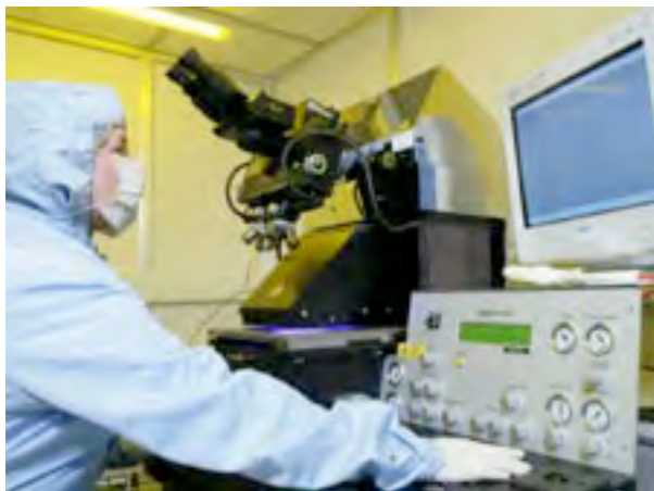
Süss MA6 optical & nanoimprint lithography
