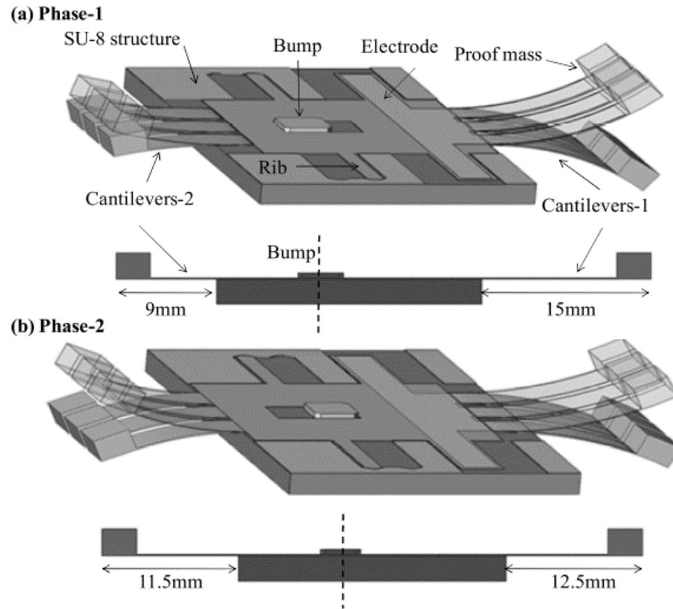
Figure 1. Schematic view of the proposed self frequency tunable energy harvester as (a)Phase-1 and (b)Phase-2
