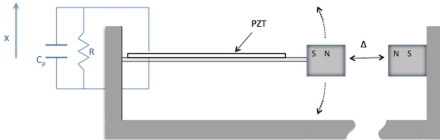
Fig. 1. Schematic of the bistable harvester considered.
