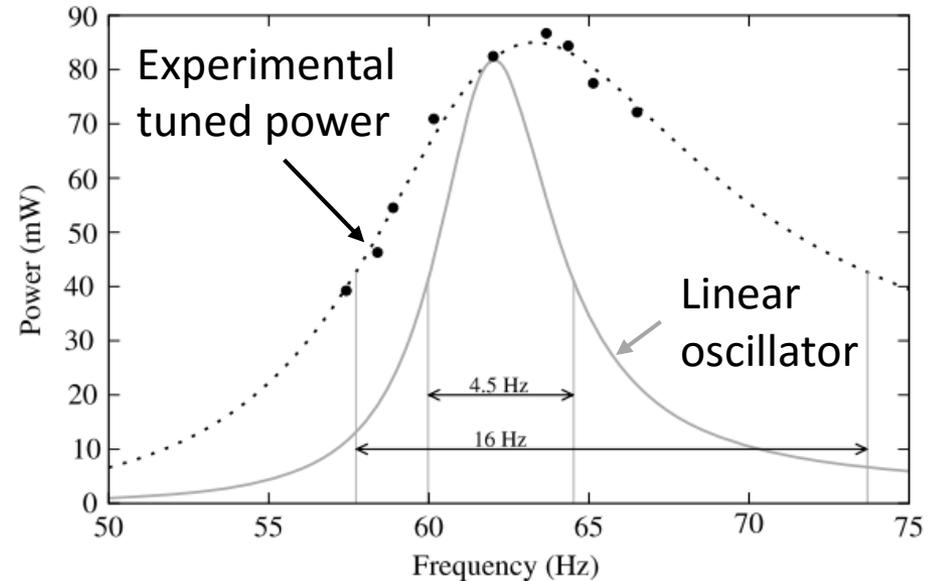
In practice the tuning range is limited by the need to produce extremely large reactive loads.
