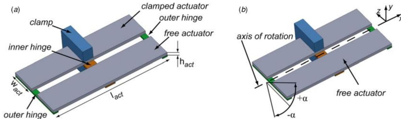
**Figure 1.** (a) Tunable resonator with one clamped and one free actuator mounted with three hinges. (b) The free actuator swings around the axis of rotation with a deflection angle  $\alpha$ .
