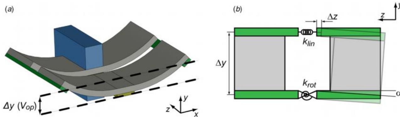
**Figure 2.** (a) Schematic cross section with applied tuning voltage. Both endings of the actuators are deflected by  $\Delta y(V_{op})$ . (b) Side view of the resonator.
