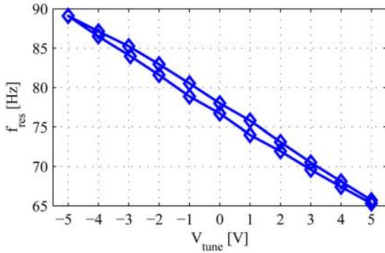
**Figure 12.** Measured resonance frequency versus applied tuning voltage (PL140).
