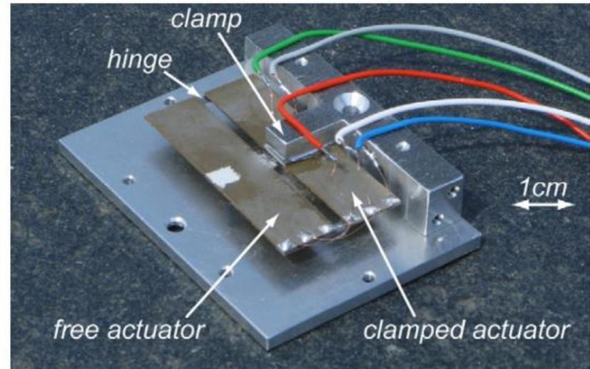
**Figure 10.** Photograph of the electrically tunable resonator with the wires for the electric tuning and the clamp support.
