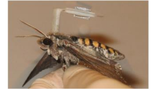
Energy harvesting from moth vibrations Chang. MIT 2013
