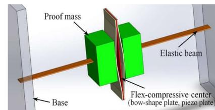
Fig. 5. Schematic diagram of the HC-PEH
