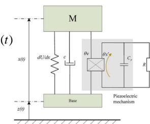
Fig. 9. Equivalent schematic of the HC-PEH with an external resistive load
