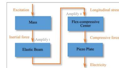
Fig. 6 Multi-stage force amplification mechanism
