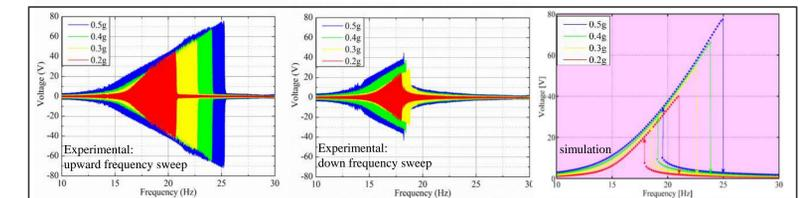
Fig. 10. Voltage responses of the HC-PEH with an optimal external resistor of 100 KΩ.
