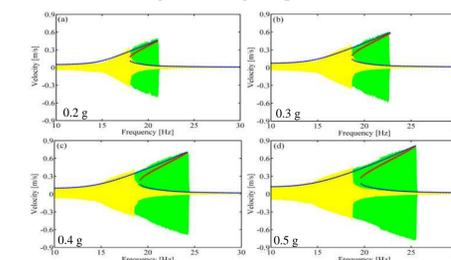
Fig. 11. Velocity responses of the HC-PEH under different excitations. The dotted lines denote simulation results and the colored regions represent experimental data.
