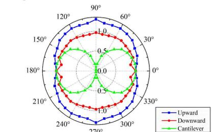
Fig. 12. Peak voltage responses normalized to the 0° voltage. The excitation direction is shifted constantly from parallel to perpendicular to the tested PEHs.
