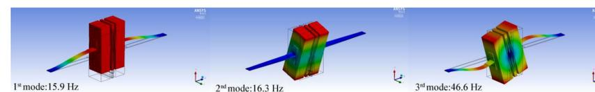
Fig. 8. Mode shapes of the first three modes from the FEM simulation
