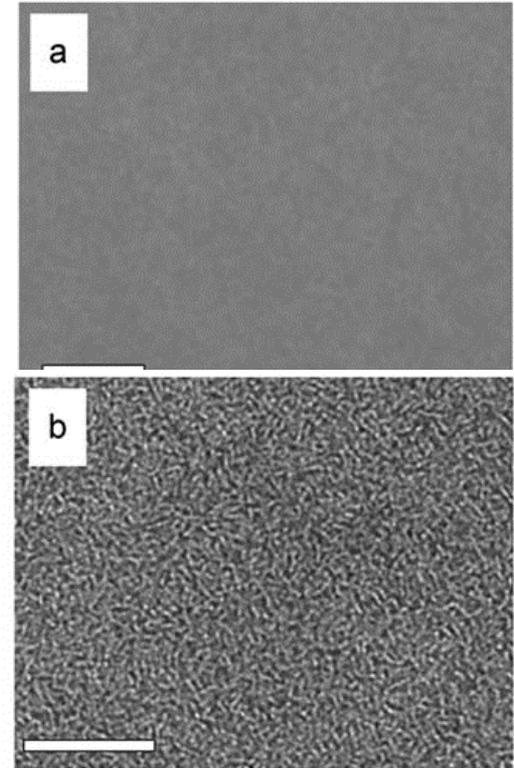
TEM images of 1:1 blend of P3HT and PCBM prior (a) and after (b) thermal annealing at 150°C for 30 minutes (scale bar 0.5  $\mu\text{m}$ ).
