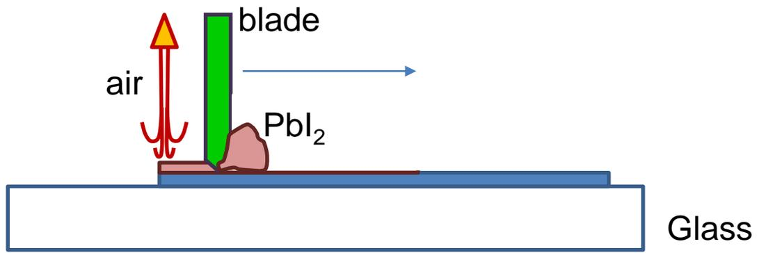
A new high performing air-assisted blade coating technique for perovskite printing
