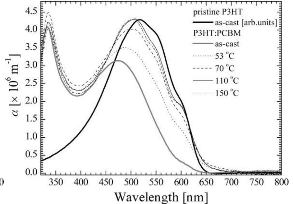
Absorption spectra of P3HT:PCBM blend films for different annealing temperatures.
