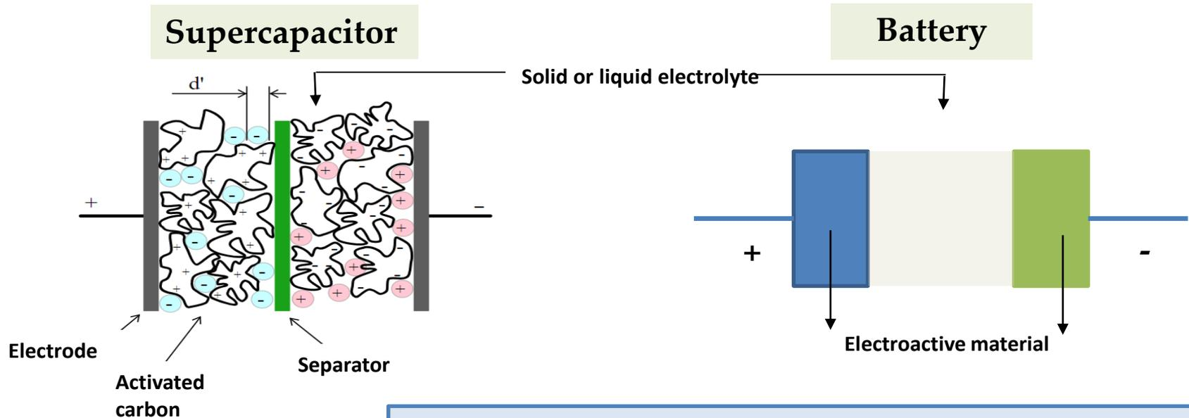
Energy storage mechanism and the similar device configuration/characterization techniques cause confusions.
