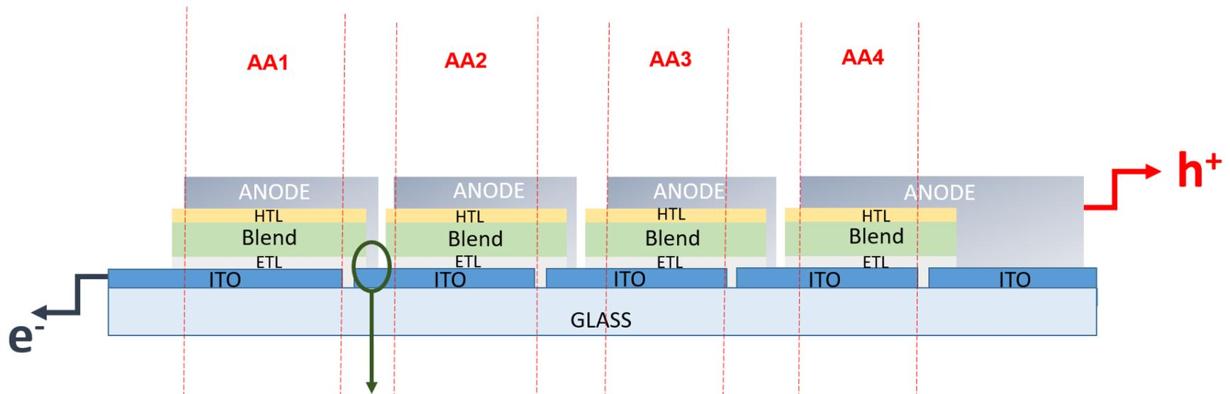
Contact between top electrode of a cell with the bottom one of the adjacent cell
