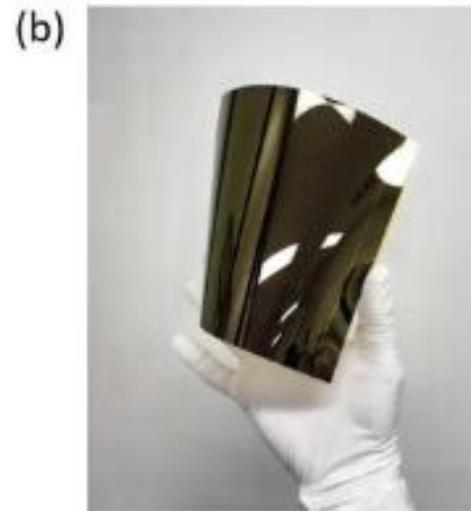
b) R2R produced flexible perovskite PV module with aperture area of 160 cm<sup>2</sup> and PCE of 10.1%.
