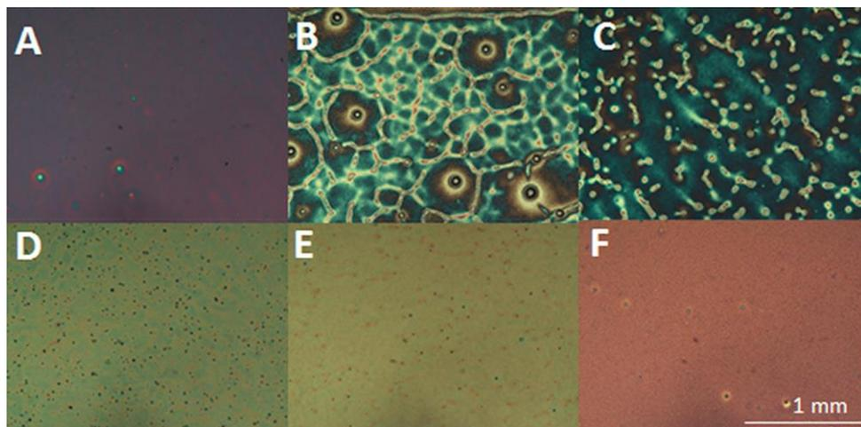
Optical microscope images of spiro-OMeTAD layer deposited from different solvents: (A) chlorobenzene, (B) anisole, (C) phenetole, (D) o-xylene, (E) p-xylene, and (F) toluene
