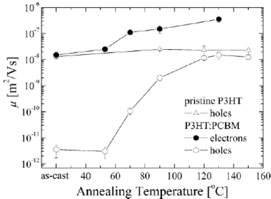
Room-temperature electron (●) and hole (○) zero-field mobilities in (1:1) blends of P3HT:PCBM as a function of postproduction annealing temperature of the completed devices. For comparison, the hole mobility measured in pristine P3HT devices ( $\Delta$ ) is also shown.
