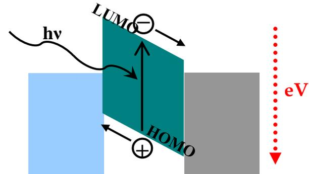
Problem: insufficient photon-current conversion (efficiency  $\sim 0,1\%$ )
