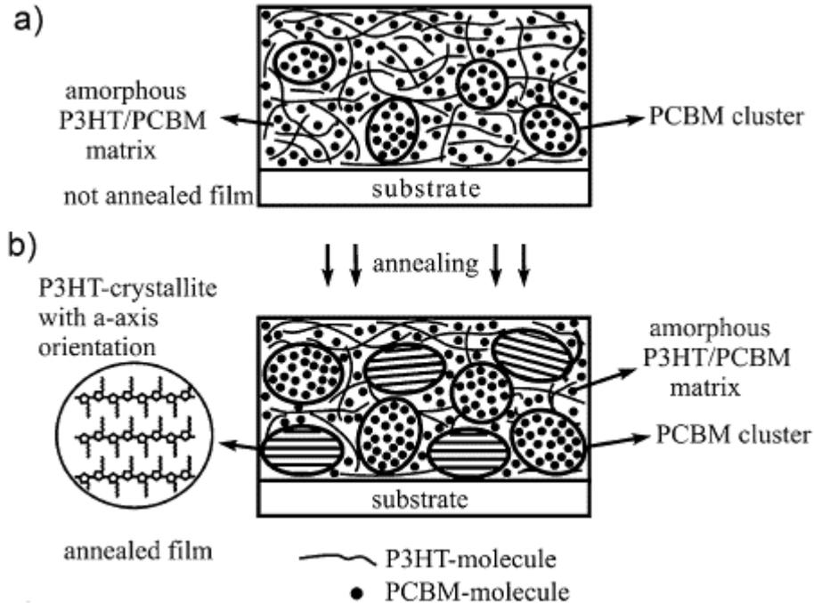
a,b) Schematic pictures showing the microscopic process during annealing. c) Grazing incidence X-ray spectrum on a blend before and after annealing, showing the evolution of the a-axis oriented P3HT crystals.
