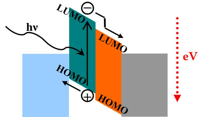
Use of two polymers, **donor** and **acceptor** (*p* and *n* type)  $\rightarrow$  better conversion efficiency ( $\sim 1\%$ )
