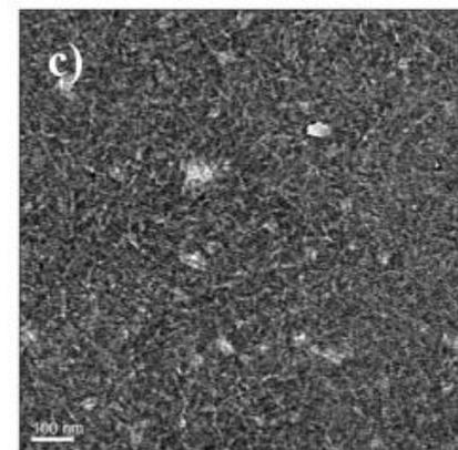
TEM image of films cast from PCPDTBT/C71-PCBM with additives: (a) none, (b) 1,8-octanedithiol, and (c) 1,8-diiodooctane
