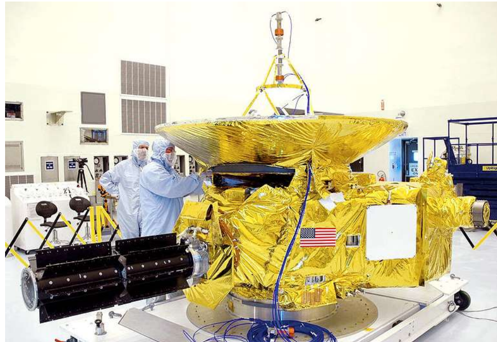
Assembly of the New Horizons probe (2005) integrating the RTG
