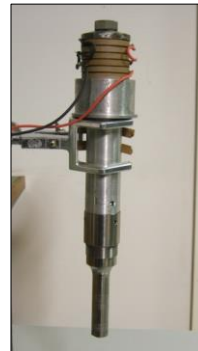
Ultrasound Generator: Horn type 750 W
